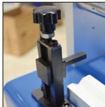
Rebar Sample Clamping
