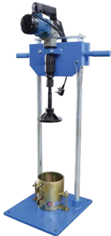
Compacting frame with Compaction Hammer
