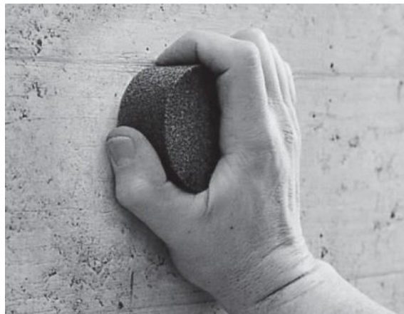
Figure 2 - Use the grindstone to smoothen the test rock surface.
