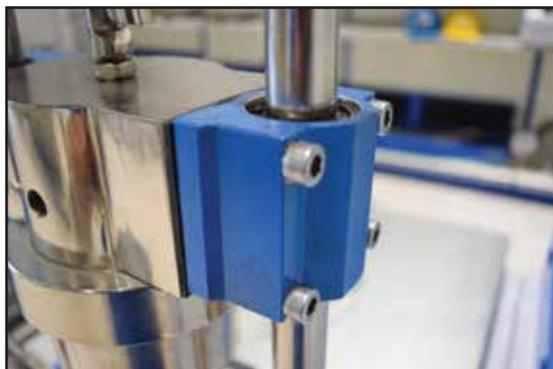
Equipped with bearing for smoother compaction drop
