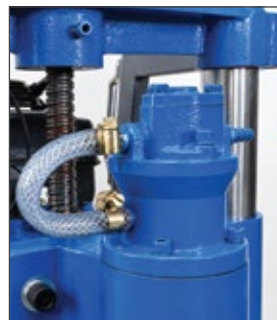
Cooling Water Suction Pump
